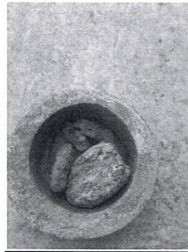
Clogged by harden ash particles (position are mostly trapped in top silo valve)
