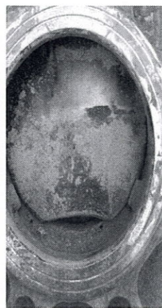
Damage seat and disc due to ash abrasion
