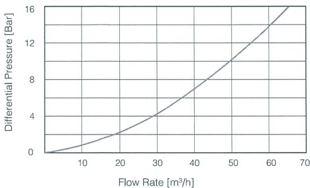
PN 16 AUTOMATIC AIR RELEASE FLOW RATE
