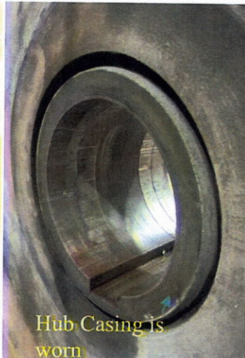
Hub Casing that contacts with bearing sleeve
