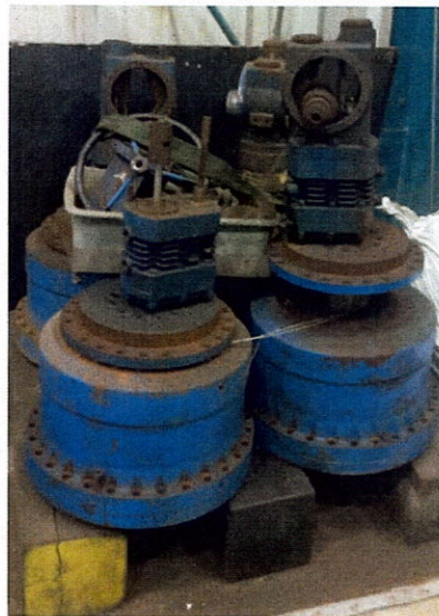
Hydraulic Vane Control Device that will be repaired
