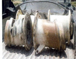
eroded plate at inlet chute
