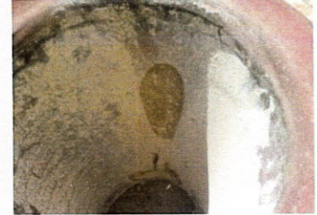
eroded plate at inlet chute
