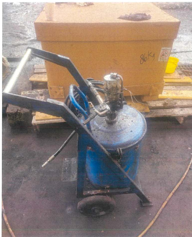
Current condition of the Grease Pump
