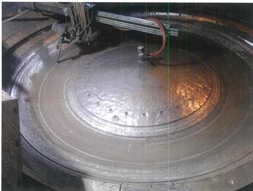
Re-welding Grinding Table
