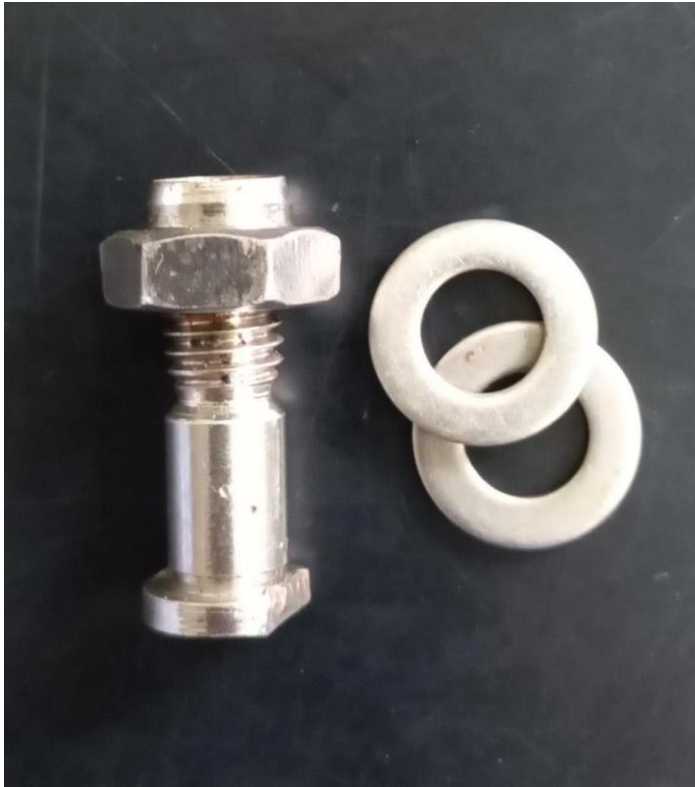
Picture item No. 20 disc pack coupling and bolt - nut
