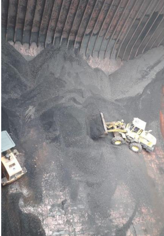
Small Wheel Loader Trimming Process in Vessel & Medium Loader manage waste material
